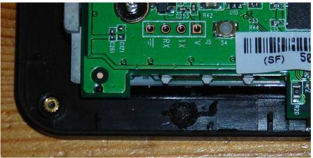
Next solder the GPS chip in as the picture below. First solder the resistors and wires to the chip and then solder it to the motherboard serial port. The wiring is the same as for the externally mounted chips.
