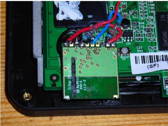
Although the chip is only in contact with the edge of the motherboard, as a precaution against shorting a piece of electrical insulating tape may be placed between the chip and the motherboard (not shown in the picture). This will also provide a little cushioning if the GPS chip is crushed against the motherboard.
