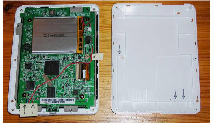
A rectangular hole is now cut as shown below. This has to be big enough such that the upper edge of the GPS chip and its wiring can sit in it when the back is fitted.
