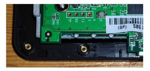
Now remove the plastic pillar and brass bush which has just been exposed. This can be ground away using a mini drill but I just nibbled it out with small sidecutters.
