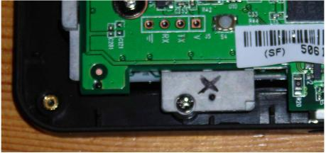
Remove the screw and then, using some small long nosed pliers bend the tab towards you so it snaps off. This should not take much force at all.
