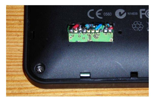
The GPS chip, resistors and wiring should not stick up above the outer surface of the inner cover so that when the outer cover is fitted they will not be crushed. When you are happy that the fit screw down the inner back cover. I stuck a piece of insulating tape over the aperture to discourage any dirt which might get under the outer cover from getting inside (not illustrated).
