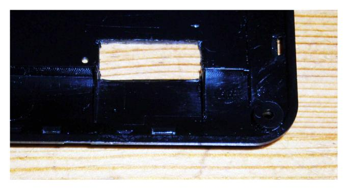
I use a scalpel for this although it can be done with a mini drill. Now carefully try the inner rear cover for fit. Jiggle the GPS chip into the the space between the webbing so that the edge of the chip and its wiring sits in the aperture you have cut. Don't force it. If it does not fit easily check to see what is jamming and correct it by trimming the cover or bending the wires.
